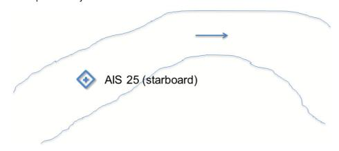
The CEVNI buoy "Bifurcation of the fairway" (without a preferred channel) cannot be encoded in the AtoN message. For the CEVNI buoys "Bifurcation of the fairway, preferable to pass on the right/left hand side" there is the same problem with right and left respectively red and green as for the buoys marking the sides of the fairway.
