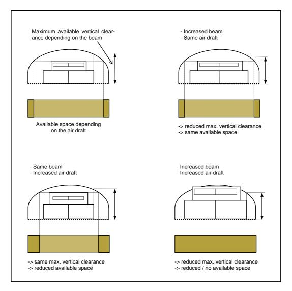
If the vertical clearance of a single bridge object of the aggregation is less than the calculated vertical clearance, this single bridge object must be symbolized by the symbol instruction "AC(CHBRN,3);TX('clr %.lf',1,2,3,'14108',1,1,CHBLK,11)"
